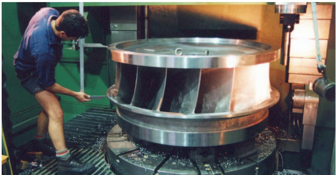
turbine is repaired with stainless steel. The turbines' outer bands are also overlaid with stainless steel before being machined back to standard on the company's CNC-controlled 6.3m vertical lathe.
